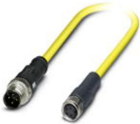
Sensor/Actuator cable, 4-position, PVC, Yellow RAL 1021, Plug straight M12-SPEEDCON, A-coded, on Socket straight M8, Cable length: 1.5 m
